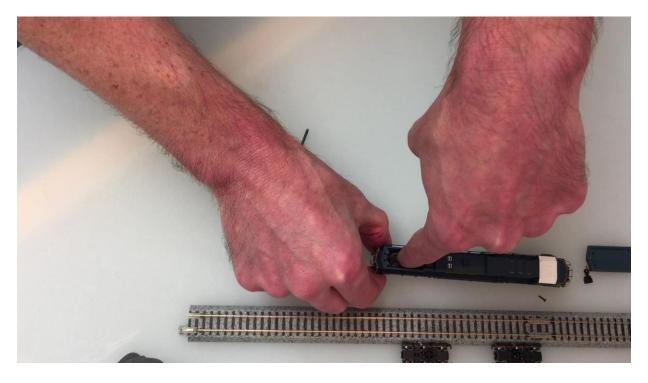
Step 5: Grasp the engine by the fuel tank, and push up on the underside of the steps on the front of the engine.
