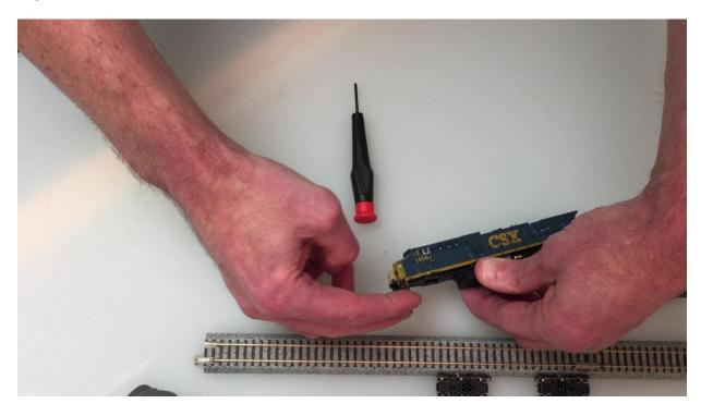
Step 6: Lift the shell away from the chassis, be aware of the cab light wires and do not pull it too far away.
