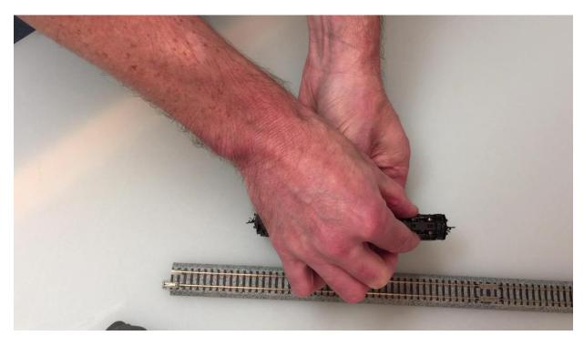
Step 2: Remove the couplers on either end (1 small Philips head screw to remove for each coupler).
